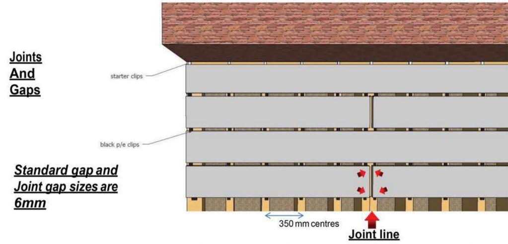
Allowing for the correct spacing of all gaps and joints is very important, like with wood and other building materials all composite decking shrinks and expands with the changes in climate. **See temperature change info and charts on pages 8 and 9**
