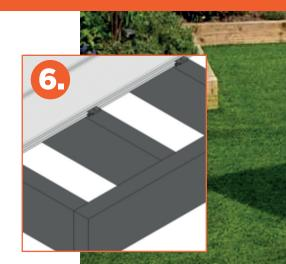
When using the T Clips and Screws lightly screw in place do not tighten at this point. (fig 3)
