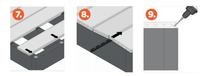
Measure the width of the last two boards with the 6mm spacing gap in between them, mark this on your last joists, using this mark install your Steel Finishing clips. Then clip your last decking board in place. (fig 7)
