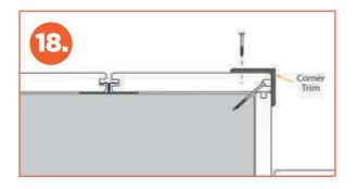
Fix the board to form both the tread and riser of your steps, installing directly onto your step framework using the T-Clip system where able to. Screw fix the exposed grooved edges or face fix the board with a composite screw (fig 17)
