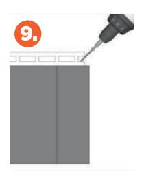
Measure the width of the last two boards with the 6mm spacing gap in between them, mark this on your last joists, using this mark install your Steel Finishing clips. Then clip your last decking board in place. (fig 7)
