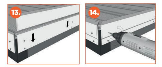
Measure the required amount of Edging trim and cut down to size, mitre down the ends at 45° angles if installing around corners (fig. 13) Cover the deck edge with corner trim and attach with screws
