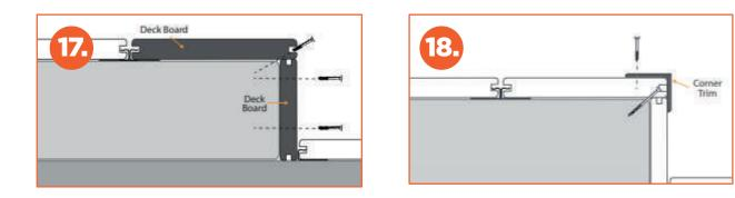
Fix the board to form both the tread and riser of your steps, installing directly onto your step framework using the T-Clip system where able to. Screw fix the exposed grooved edges or face fix the board with a composite screw (fig 17)
